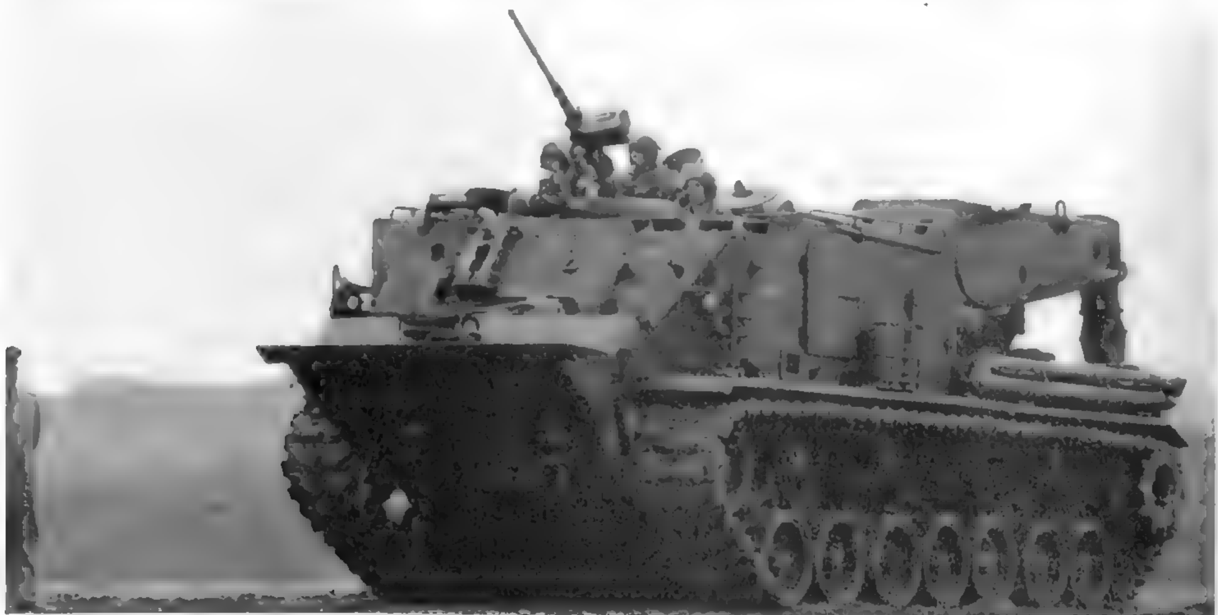
The M51 was a massive vehicle. The front anchor spade is visible, as is the sheave mounted on it for use in recovery operations. One advantage of its massive size was its ability to climb a 36-in. vertical wall. Just behind the fuel cans on the retriever's side is the heavy-duty tow bar. (Photo courtesy of the Patton Museum)
